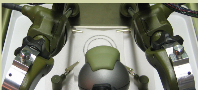
SENSORS TRACK TIME, PATH, ROTATION, AND FORCE
